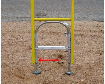
**4.** Install Angle Rites to inside or outside of ladder rails, according to Angle Rite instructions. Be sure to read Angle Rite instructions provided prior to installation. View bubble level to confirm ladder is at proper 75.5° angle. Adjust ladder until bubble level is
